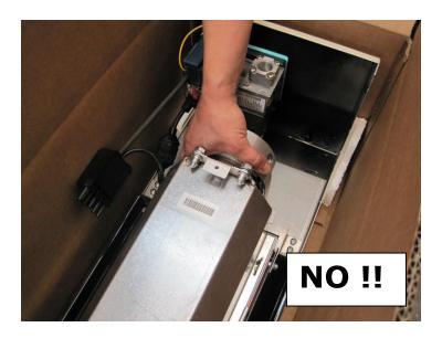
Appliances must be taken at the installation point / height inside its package or <u>using M8 inserts</u>: all other parts of the appliances are NOT designed to withstand its weight.
