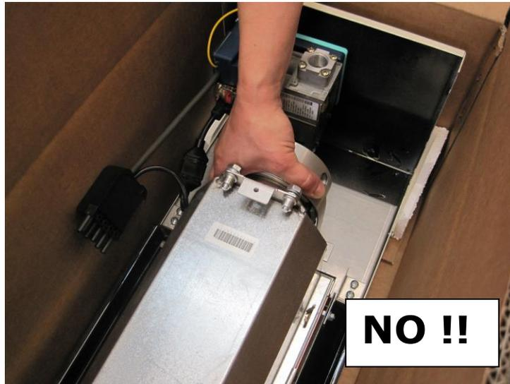
Appliances must be taken at the installation point / height inside its package or using M8 inserts: **all other parts of the appliances are NOT designed to withstand its weight.**
