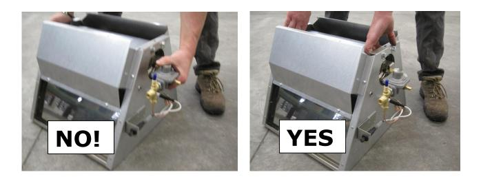
Appliances must be taken at the installation point / height inside its package or <u>using M8 inserts</u>: **all other parts of the appliances are NOT designed to withstand its weight.**
