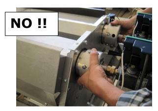
Appliances must be taken at the installation point / height inside its package or <u>using M8 inserts</u>: **all other** parts of the appliances are NOT designed to withstand its weight.
